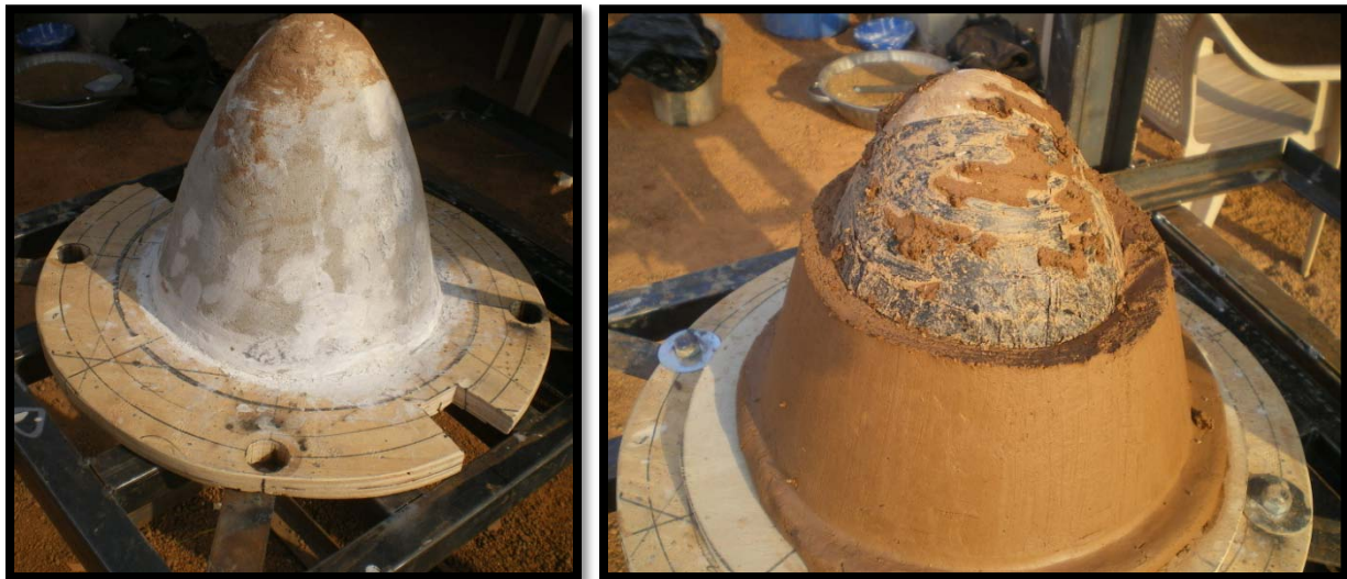
Left: Male Mold on Table , Right: Male Mold, Plastic Bag and Test Filter, Cut in Half
