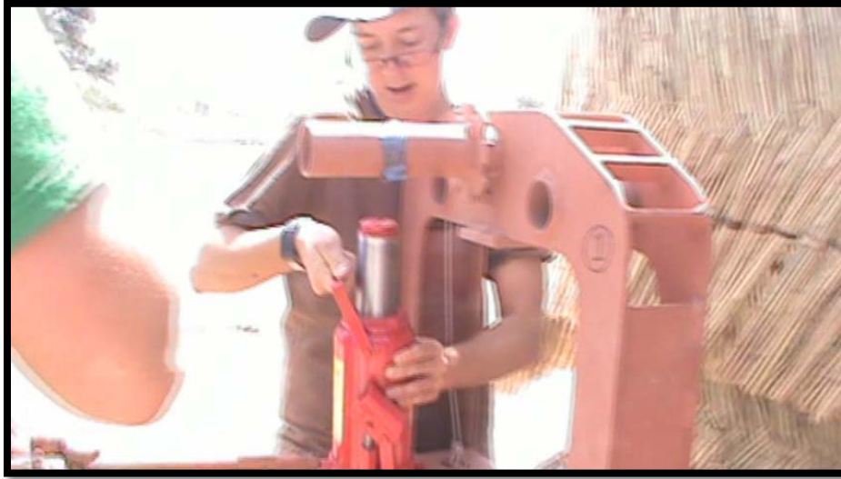
Removing 20-Ton Hydraulic Jack from the Press Just After the Valve is Opened
