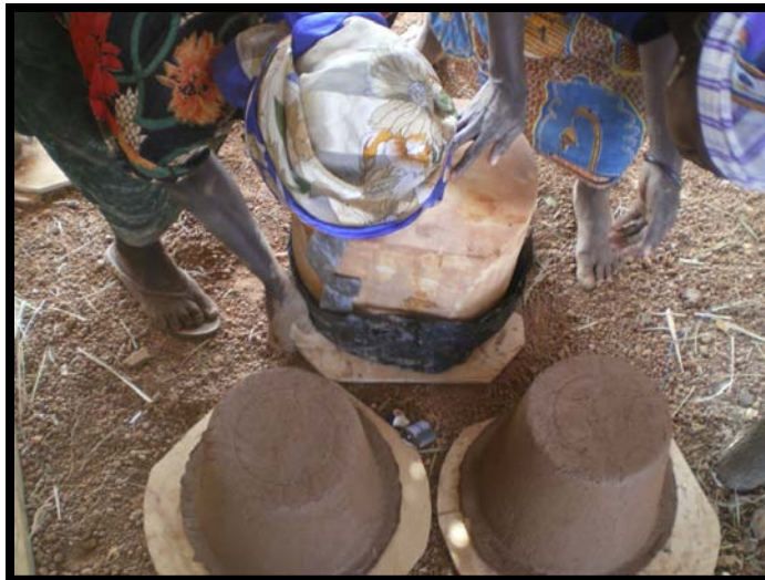
Lifting the Female Mold off the Newest Filter
