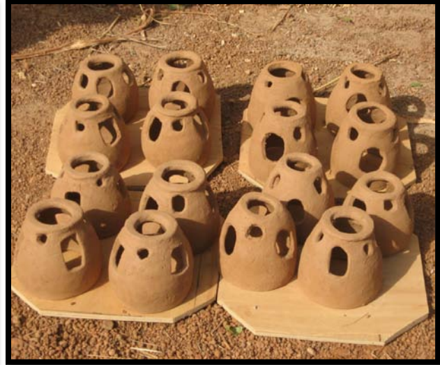
Left: Potter Crafting the Ceramic Spacer, Right: Fired Ceramic Spacers (More Holes to be Added to the Top)
