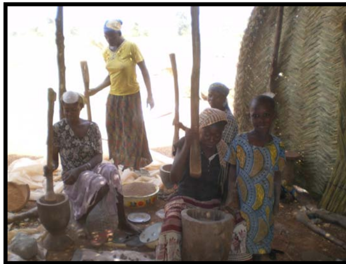
PHW Employees Grinding Dry Clay with Wooden Mortar and Pestles
