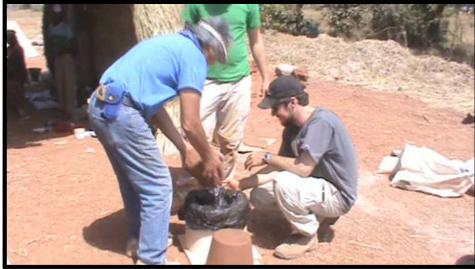
Placing 8.5 kg Cube of Clay Mixture into Female Mold with Wetted Bag Inside
