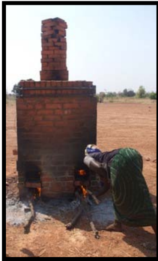
Tending a Small “Candle” Fire in the Lower Firebox for Four Hours
