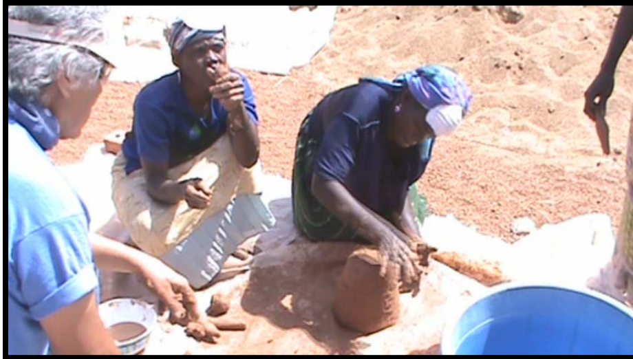
Forming 8.5 kg of Clay into Roughly a Cube
