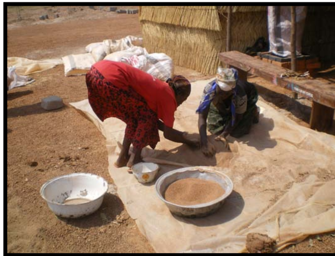
Dry-Mixing the Clay, Grog and Rice Husk Mixture on a Tarp
