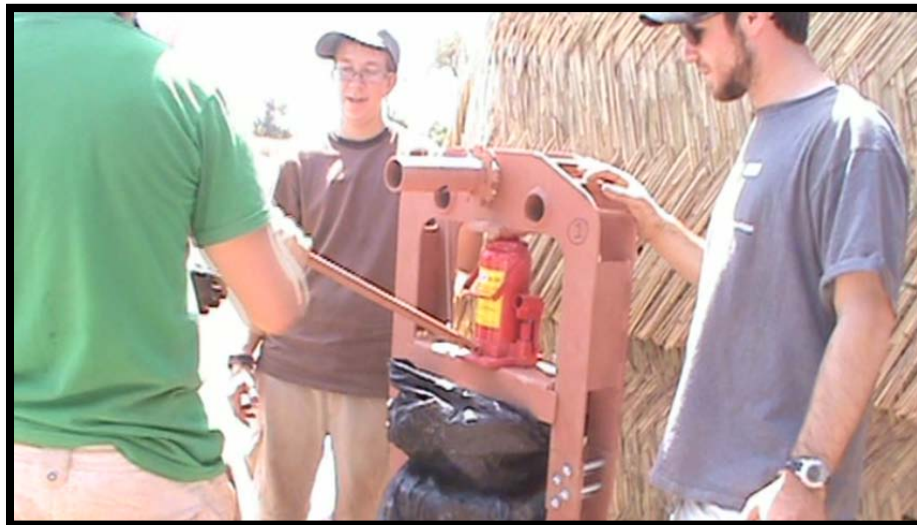
Turning the Valve at the Base of the Hydraulic Jack using the End of the Crank
