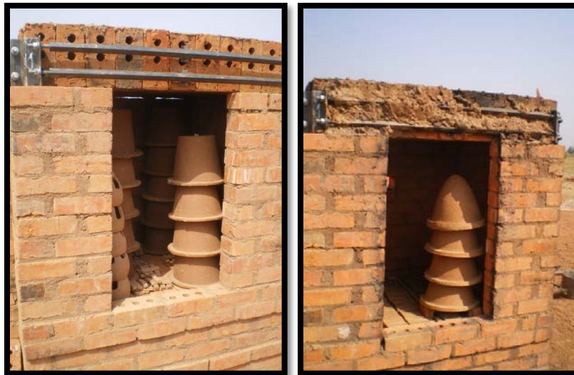
Flower Pot Filters (Left) and Paraboloid Filters (Right) Stacked for Firing in Kiln
