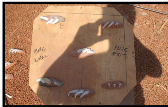
Cone Packs Arranged to Represent their Relative Position inside the Kiln
