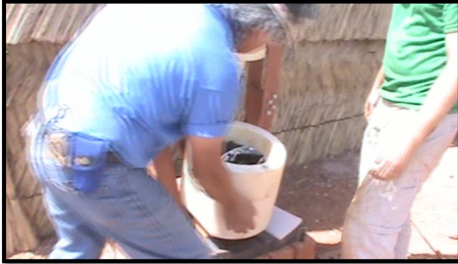
Returning the Female Mold to the Press
