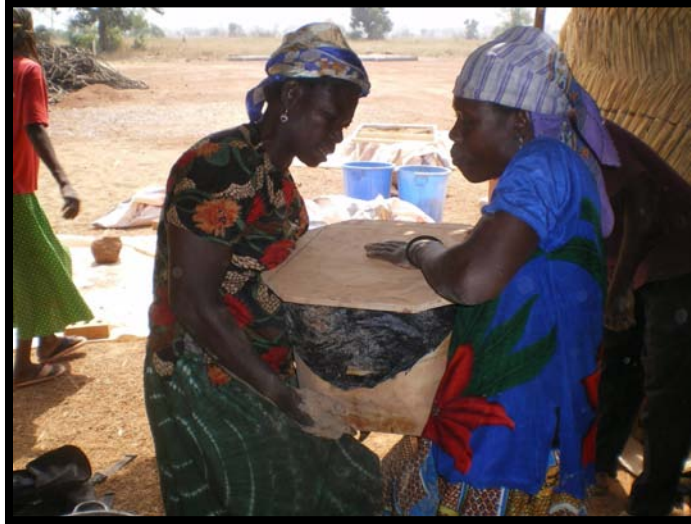
Inverting the Female Mold with the Plywood Bat on Top
