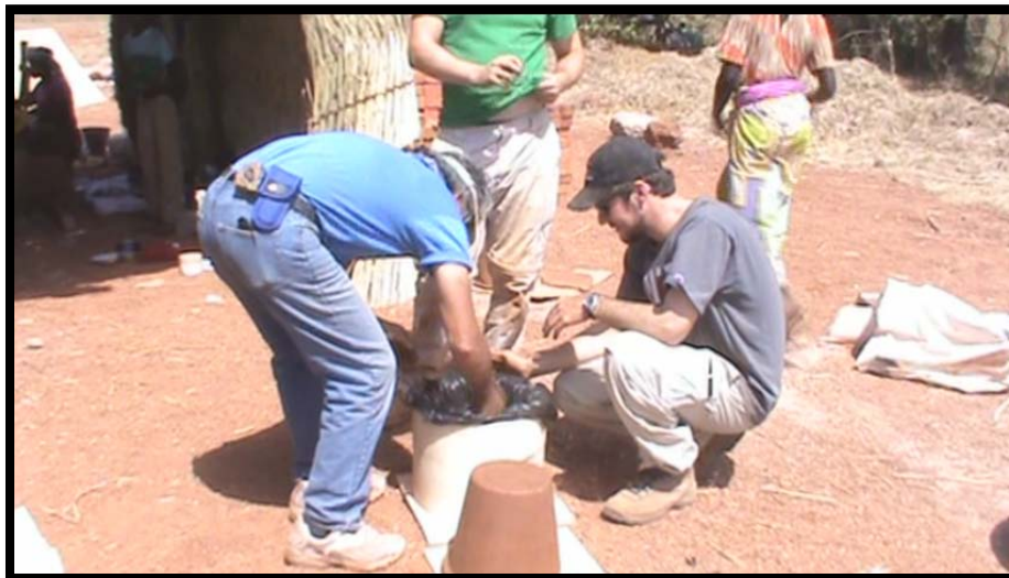
“Punching” the Clay with a Fist to Create an Even Depression
