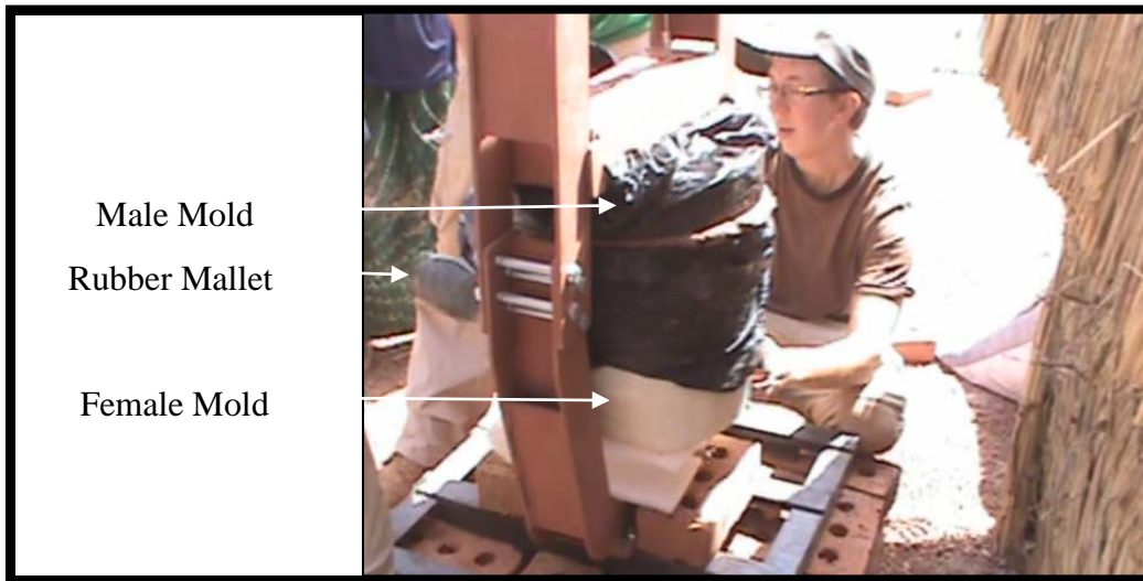
Striking the Female Mold to Encourage the Molds to Separate
