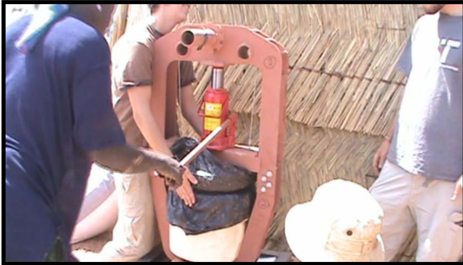
Pumping the Hydraulic Jack to Push the Male Mold into the Female Mold
